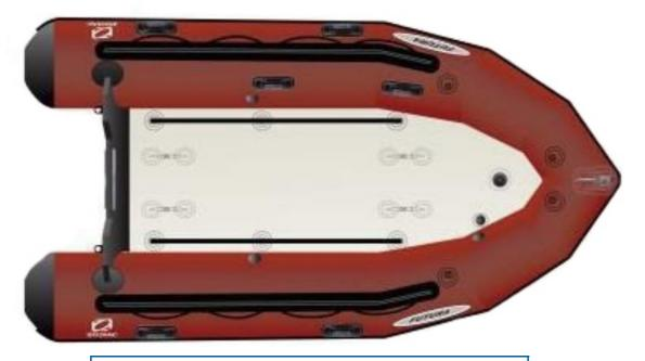
HULL & DECK: 2 bailers, 2 Towing rings.
